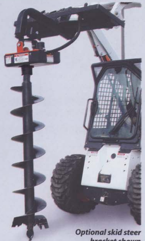
BUCKET MOUNT POWERHEAD (185 lbs with quick attach)
