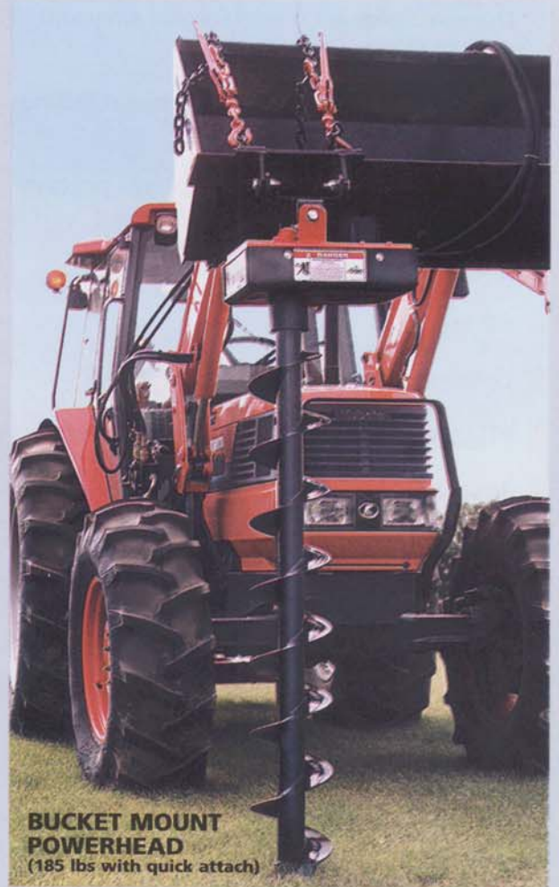
Choice of bits in 4", 6", 9", 12", 15" diameters with 3', 4' or 5' extensions
